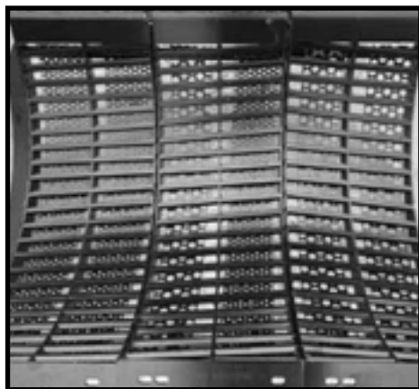
Angled bars, in different directions, improve thrashing
